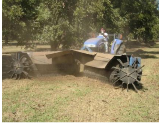
Fig. 15 - "V" side sweeper used to windrow crop
