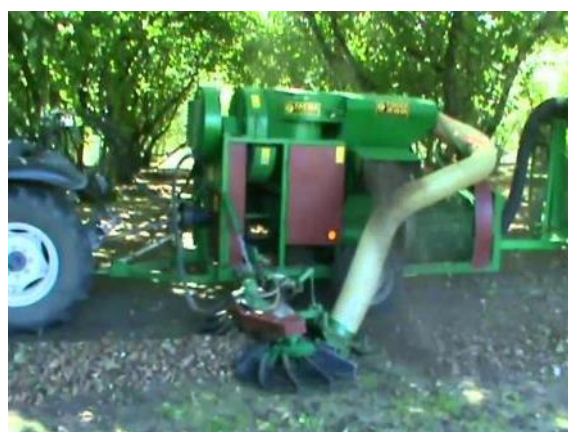
Fig. 16 – Tractor-towed vacuum harvester with side-mounted, sweeper assisted pickup
