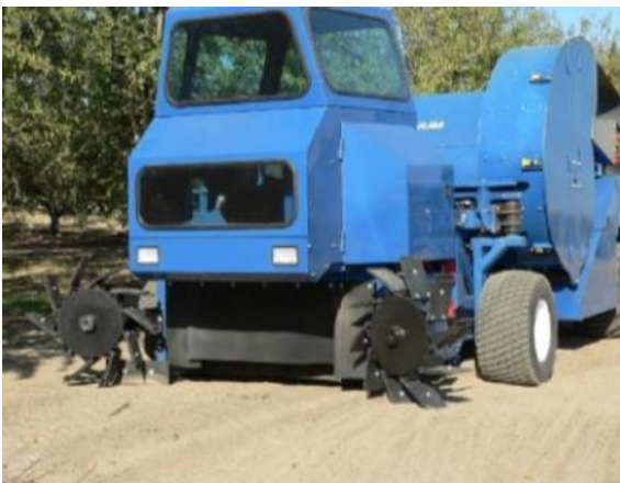
Fig. 3 - Self-propelled mechanical harvester designed for bare ground
