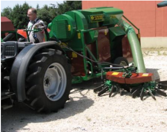
Fig. 7 - Tractor mounted PTO driven Facma vacuum harvester
