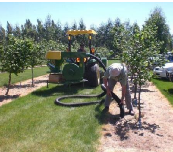
Fig. 9 – Small tractor mounted Chianchia harvester
