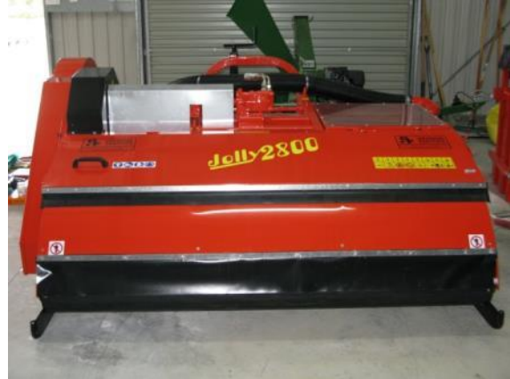
Fig. 10 - Tractor mounted PTO or hydraulically driven Jolly mechanical harvester
