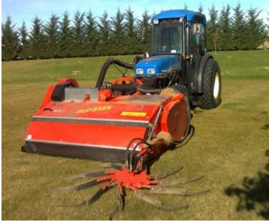
Fig. 10 - Tractor mounted PTO or hydraulically driven Jolly mechanical harvester
