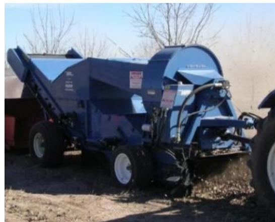
Fig. 13 - Towed mechanical harvester designed for soil cover
