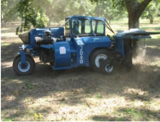
Fig. 14 - Straight side sweeper used to windrow crop
