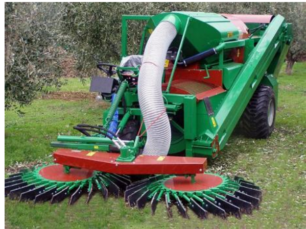
Fig. 10 - Tractor mounted PTO or hydraulically driven Jolly mechanical harvester
