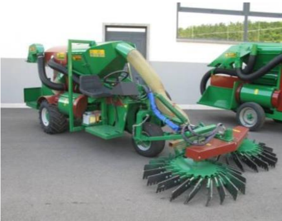
Fig. 8 - Self-propelled Facma vacuum harvesters
