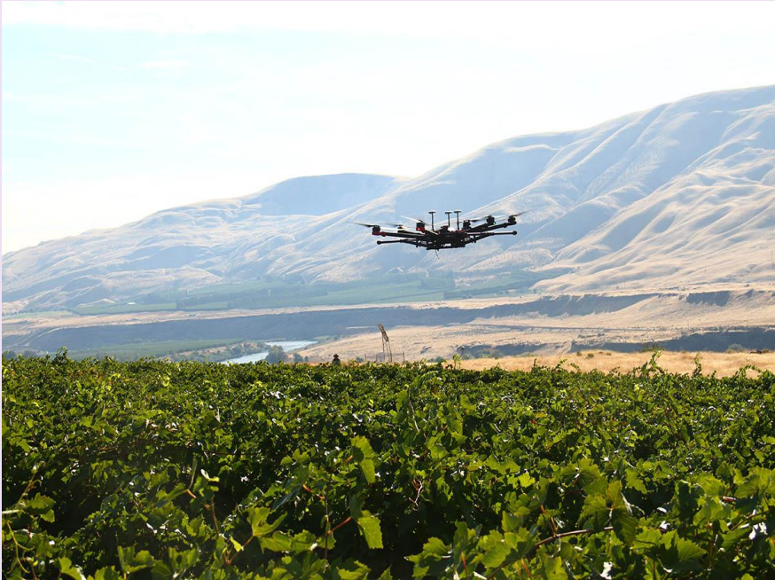
A manually operated WSU drone flies over a vineyard during tests for bird deterrence and fruit damage assessment. Credit: WSU Agricultural Automation and Robotics Lab
