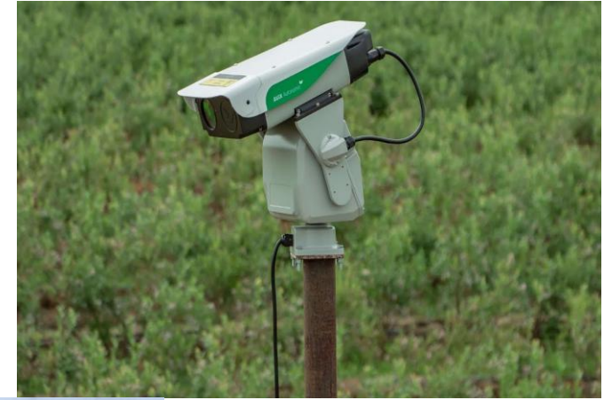
AVIX Autonomic Mark II, Bird Control Group - example of a fully automated laser bird repellent. Image: Bird Control Group
